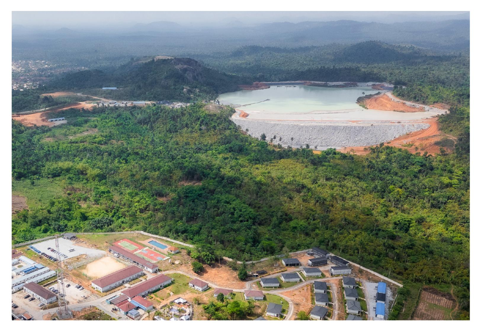
Tailings from the processing plant are hydraulically transported as a slurry to the engineered Tailings Management Facility (TMF), a critical containment structure designed and rigorously managed to ensure long-term dam stability and prevent environmental seepage.
