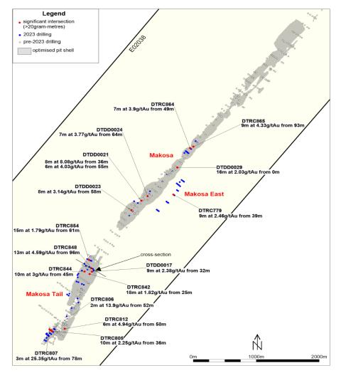
Figure 2.6 Drillhole location map showing Significant Results (>20gram-metres)
